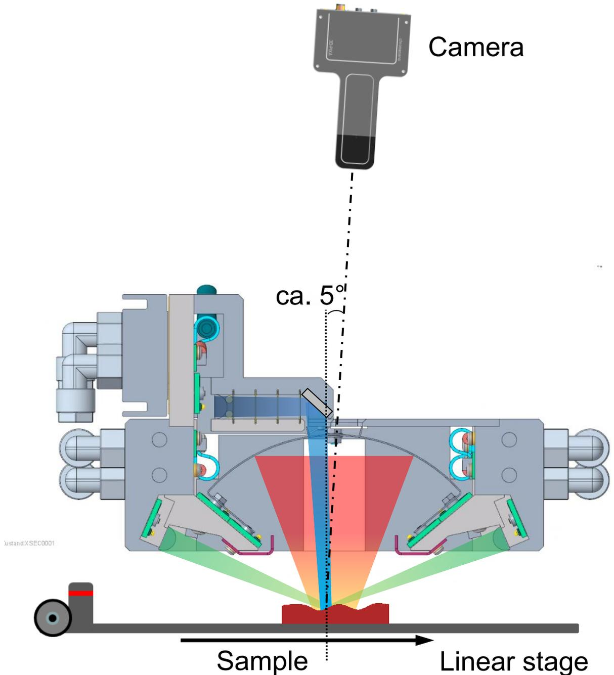
The tube illumination (diffuse light) is used to illuminate the balls of the BGA over a large range of angles. The diffuse light illuminates the balls homogeneous from every direction. This ensures the best 3D data reconstruction of the ball surface from the stereoscopic image data.
