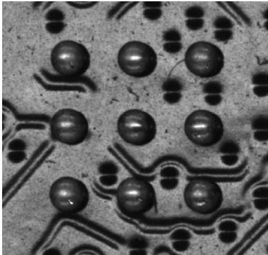
A further aspect of the image acquisition is the noise level of the image. A noisy image reduces the quality of the 3D reconstruction especially in darker image regions, parts with a weak texture and parts that are far away from the working distance.
