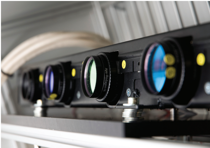
FIGURE 1. Color printing processes can be monitored in real time using a 12-channel spectral linescan camera system from Chromasens. The system, which uses four RGB linescan cameras, can be mounted on a printing press to monitor color fidelity with high accuracy.
